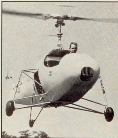
The first of three experimental Model 30s, NX41867 was the first full-scale flying application of Arthur Young's stabilizer bar.
